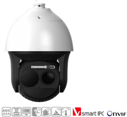
PB-T26450-Z 36XThermal & Optical Bi-spectrum Network Speed Dome use a vanadium oxide uncooled focal plane sensor to enhance thermal image quality. The high sensitivity sensor has 640 × 512 resolution and features contrast adjustment for optimized images. AGC (Automatic Gain Control), 3D DNR (Dynamic Noise Reduction), and Dynamic Detail Enhancement further enhance image quality.
