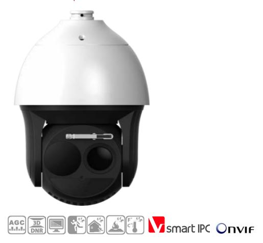
PB-T23850-Z 36x Thermal & Optical Bi-spectrum Network Speed Dome use a vanadium oxide uncooled focal plane sensor to enhance thermal image quality. The high sensitivity sensor has 384 x 288 resolution and features contrast adjustment for optimized images. AGC (Automatic Gain Control), 3D DNR (Dynamic Noise Reduction), and Dynamic Detail Enhancement further enhance image quality.
